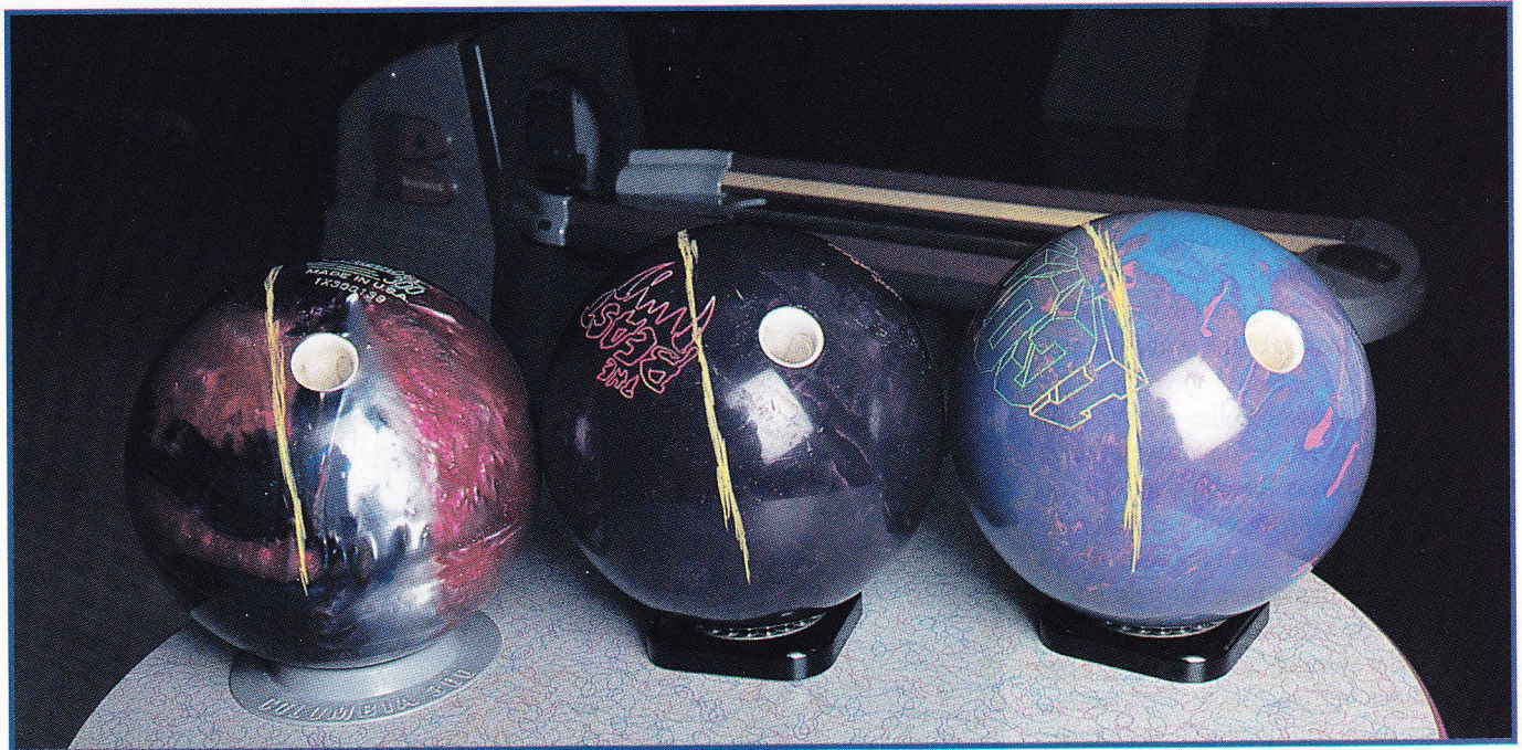
Oil tracks are marked on a pancake-block low-flaring core [left], a two-piece low-flaring core [center], and a multipiece high-flaring core.
